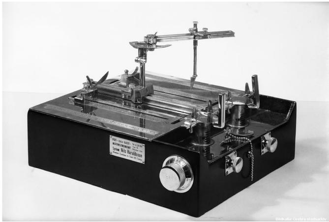
**Figure 5** Foot measuring apparatus in detail. Foot measurement apparatus developed by Nils Haraldsson and used by the Swedish Shoe Industry's Research Institute. Between 1940-1990, the feet of 16,000 people in Sweden were measured. Photographer Curt Götlin 1951/Örebro stadsarkiv. Homepage available 2016-04-22 The apparatus can be seen at the Kumla Skoindustri Museum.
